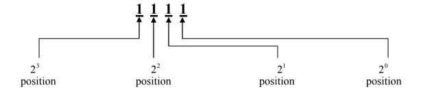
Note that the most significant bit position is the  $2^3$  position. If we add 1 to this number (and ignore the fact that overflow will occur), the result will be 10000. Converting this to decimal is easy: There is only a single 1 in the  $2^4$  position. So, one number larger than 1111 is equal to  $2^4$ . So 1111 must be equal to  $2^4-1$ .
